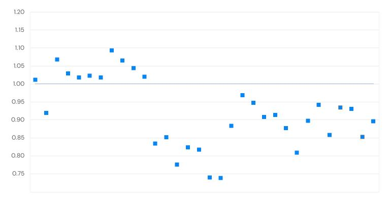
Figure 2. Weather-corrected production normalized by P50 pre-construction energy estimate for 32 wind farm years.
