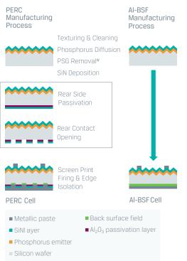
(Left) The PERC Cell design and manufacturing process. (Right) The Al-BSF cell design and manufacturing process. (box) Extra process steps associated with the PERC cell. \*The phosphosilicate glass ("PSG") removal step needs to be optimized specifically for PERC to planarize the rear of the cell.
