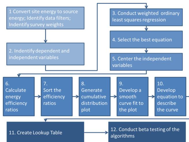
Figure 5 – Steps to Develop a Building Energy Performance Benchmarking Tool
